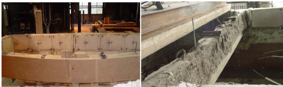
Figure 15 NSC and HSC beams at failure [20]
