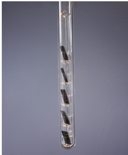
Figure 1.4: Special construction enabling the oxidation of a set of am- \text{Al}_x\text{Zr}_{1-x} specimens with various alloy compositions under identical oxidation conditions.
