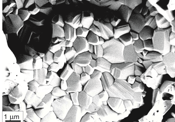
Figure 12: SEM micrograph of the cross-section of a microcrystalline sample upon sintering at 1700 °C for 8 hours.
