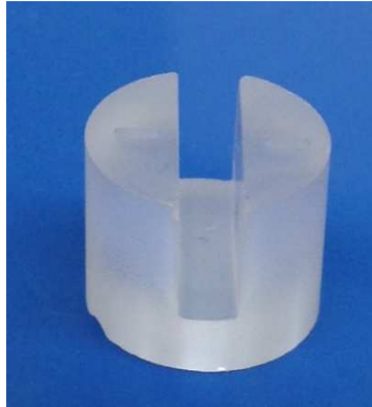
Figure 9: Sapphire sample holder specifically designed to reduce the spurious contribution to the impedance spectroscopy measurement.
