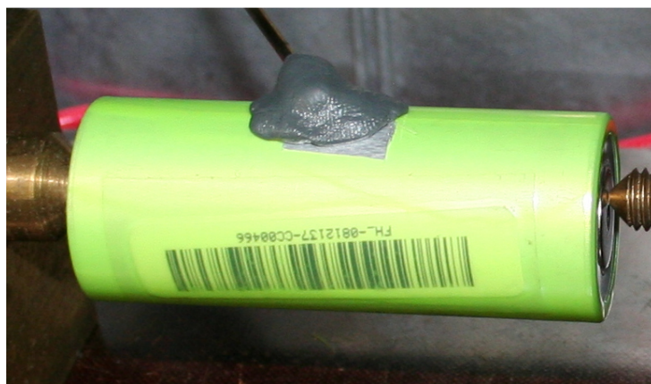
Figure 5.3: Thermocouple fixed at the center of 26650 cell surface. Patch of plastic cover was removed to measure temperature at the metal surface.
