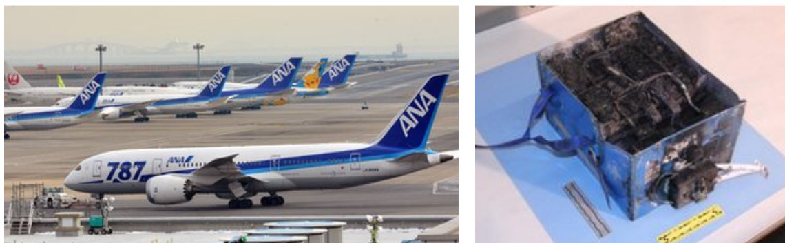
Figure 2.16: Boeing 787 Dreamliner (left) and battery pack removed from ANA flight for inspection (right) [61].
