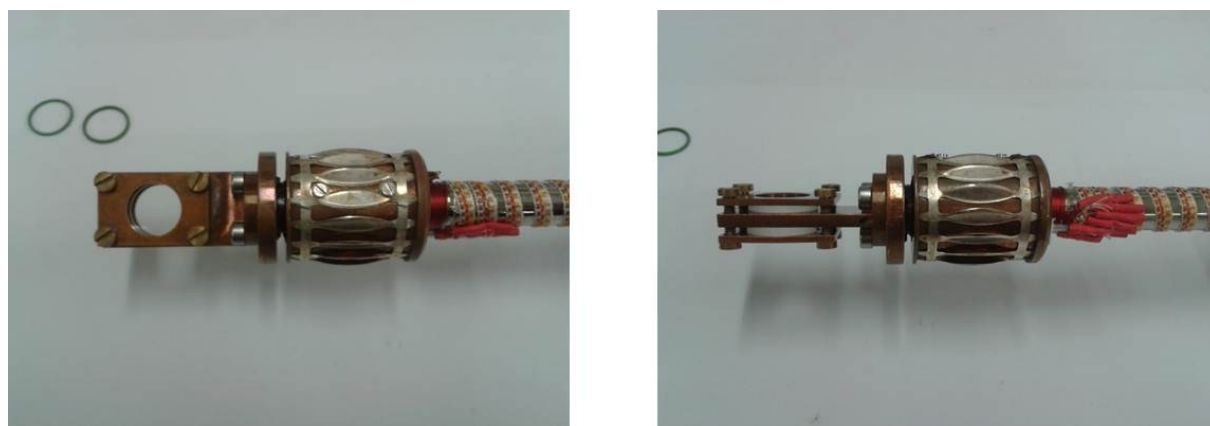
Figure 25: Home-built sample cell screwed to the sample rod. Fused silica disks are attached to both sides of the middle part. Left: Top view. Right: Side view.
