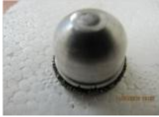
Figure 4-39 View of the brush projectile from the top side (EX04)
