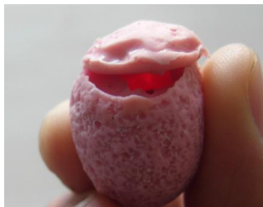
Figure 4-18 Torn P05 projectile after being stuck and released
