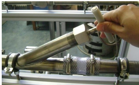
Figure 3-11 Projectile insertion assembly
