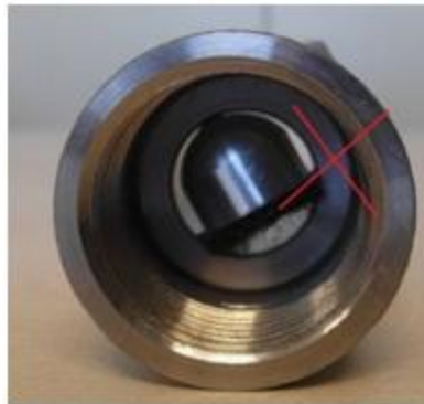
Figure 4-40 Projectile gets stuck while trying to pass horizontally through the reducer
