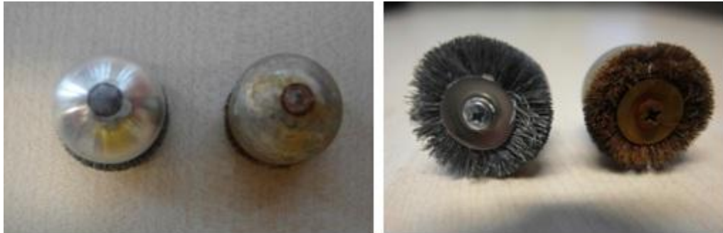
Figure 4-45 Projectile EX04 before (left) and after (right) one day of experiment
