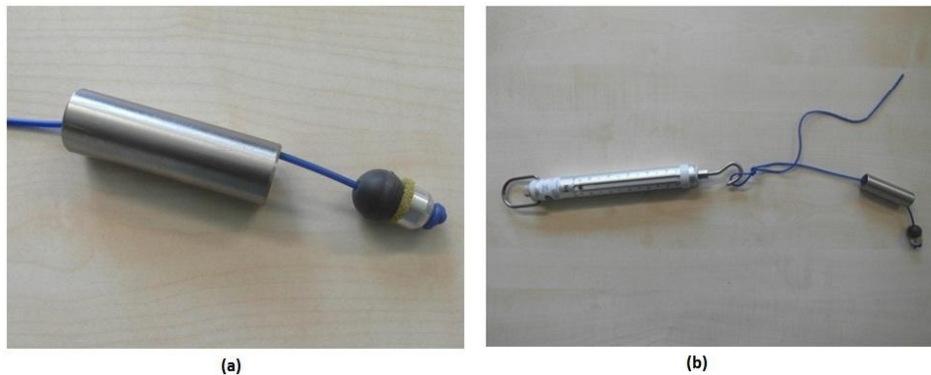
Figure 4-48 Tensometer to measure the required force to pull the projectile through the tube
