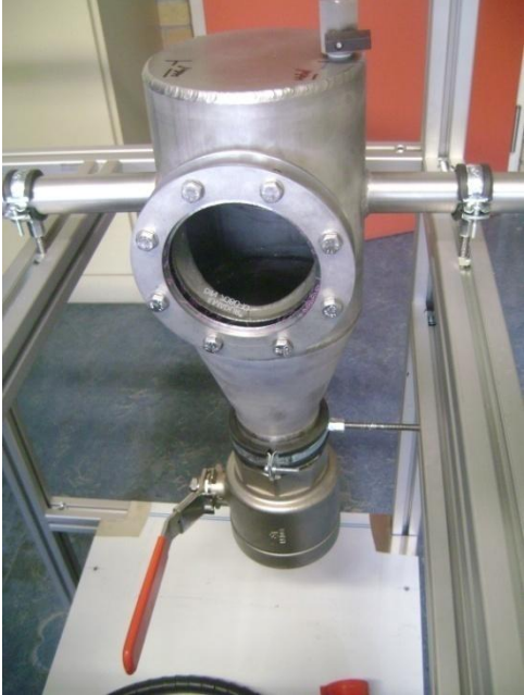
Figure 3-9 A picture of the projectile collector
