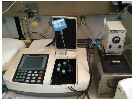
Figure 7: Experimental setup to determine the temperature dependence of the reaction rate of S-IRED-Pe.
