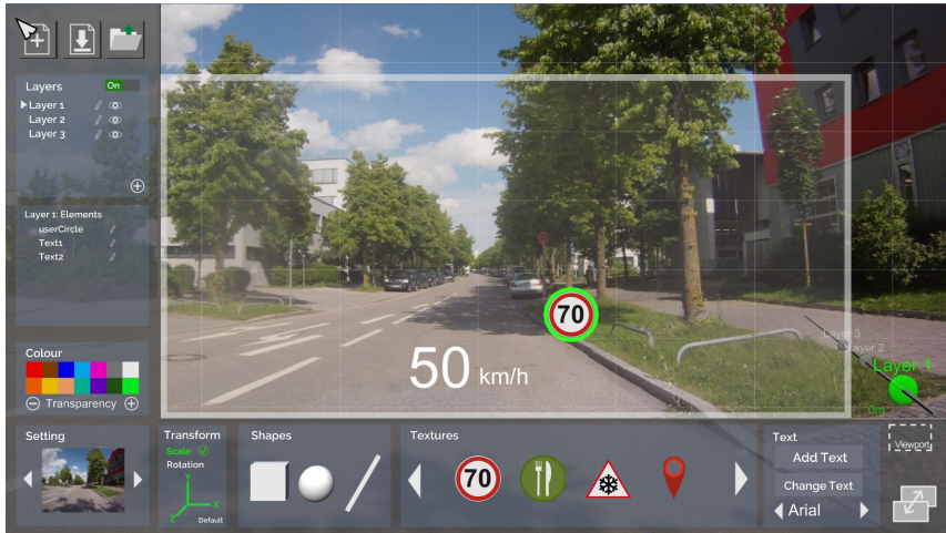
Figure 7.8: The S3D-HUD Designer allows the user to create the spatial layout of a HUD in front of a static 3D scenario.
