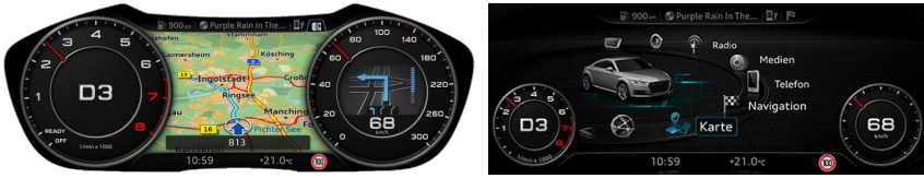
Figure 3.3: Audi’s virtual cockpit provides a classic (left) and infotainment view (right) in its instrument cluster (pictures taken from website 11 ).
