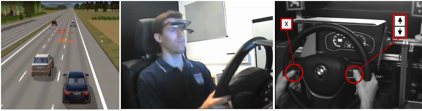
Figure 8.4: For the primary task the participants followed a white vehicle on the right lane (left picture). We tracked the gaze behavior while driving (middle picture). For the secondary task (right picture) a button ‘X’ on the left side of the steering wheel needs to be pressed for judging the position of symbols. A toggle button (‘↑’ or ‘↓’) on the right side of the steering wheel decodes the reaction on unexpected events.
