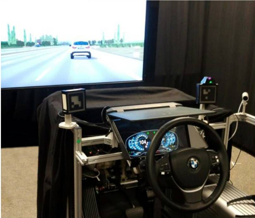
Figure 8.1: We used a mid-fidelity driving simulator to evaluate the influence of a 3D visualization, the display technology, and the interface complexity on user performance and subjective perception.
