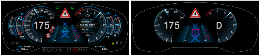
Figure 8.3: The left image depicts the high complexity layout of the IC while the right picture shows the low complexity layout.
