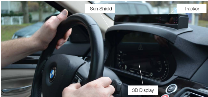
Figure 9.1: We replaced the IC of a car with an autostereoscopic display technology using eye tracking to adjust the sweet spot.
