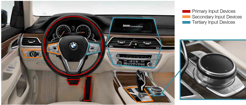
Figure 3.1: We can classify the vehicle controls in accordance with the primary, secondary, and tertiary task (based on [143,233]).
