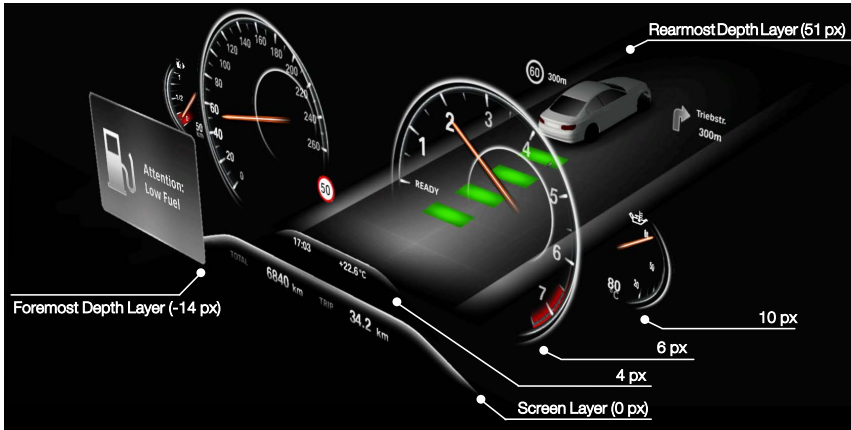
Figure 9.3: Side view of the IC showing the depth layout of the UI elements as parallaxes in pixels.
