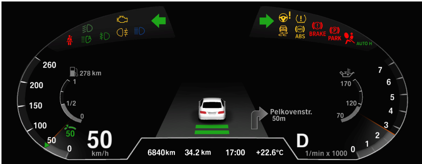
Figure 9.9: The IC places speed, rpm, check controls, and status information at the outer edge to clear space for elements which can profit from a 3D representation as, for example, Active Cruise Control.
