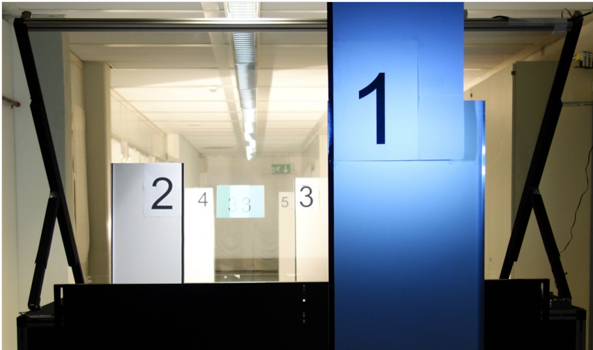
Figure 5.16: The setup of the depth judgment study shows a numbered virtual object through a see-through display and several real world shields.
