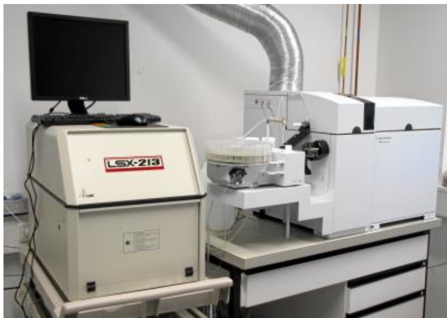
Fig. 3.8. Laser-ablation inductively-coupled plasma-mass spectrometer (LA-ICP-MS) combining a Cetac LSX-213 system with an Agilent 7700s ICP-MS (from: http://www.uni-stuttgart.de/imi/institut/ausstattung.html ).
