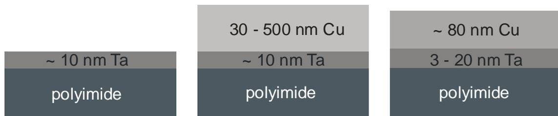
Figure 5.1: Schematic drawing of the Ta and Ta-Cu film systems investigated. The Ta as well as Cu film thickness was varied.
