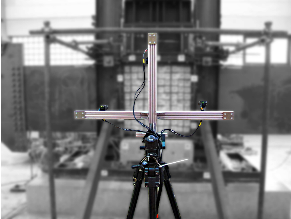
Figure 3.2: Placement of cameras for photogrammetric measurements.
