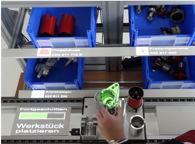
Figure 6.4: The projected feedback can be enhanced with additional information. In the beginner level, a video is shown additionally to text, image, and contour feedback. In advanced level only the contour is shown. In expert level, no visual feedback is shown at all.
