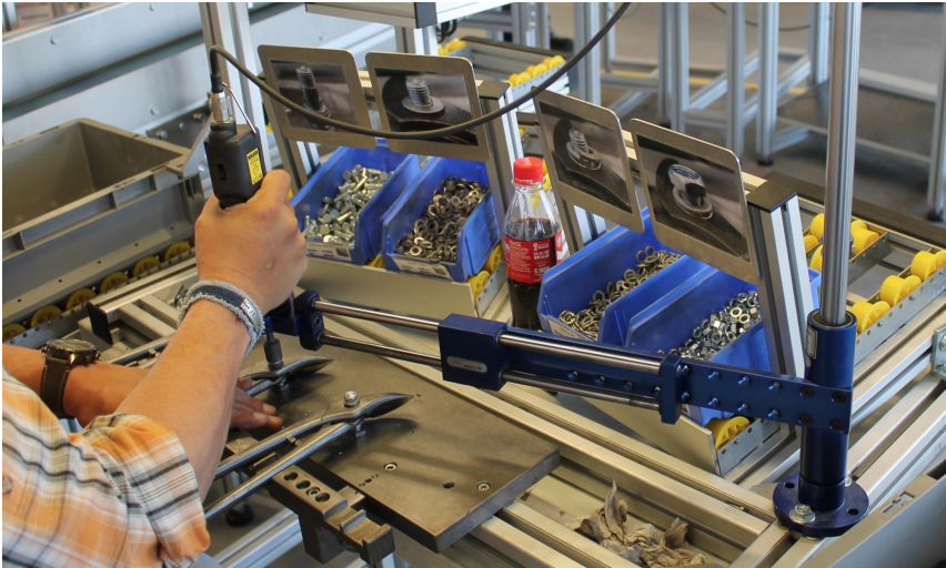
Figure 8.6: A state-of-the-art assembly workplace that is used in the analyzed sheltered work organization. Pictorial instructions above the bins holding the parts to assemble show how the assembly has to be performed. Workers can compare their assembled product with the depicted instruction.
