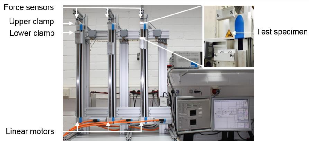
Figure 84. Self-developed testing facility for mechanical fatigue testing of thin silicone films.
