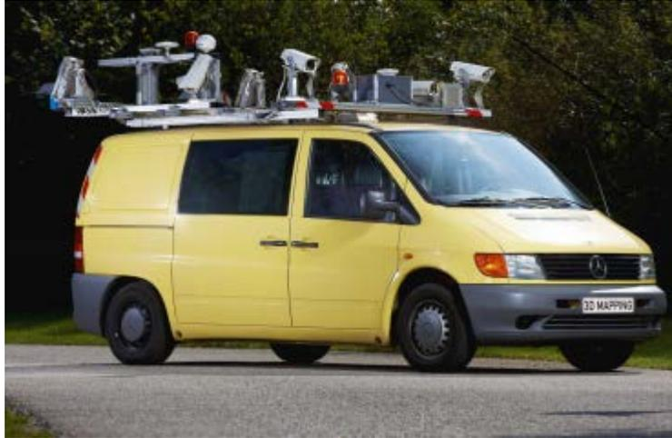
Figure 6.2: MoSES mobile mapping system (3D-MAPPING 2014).
