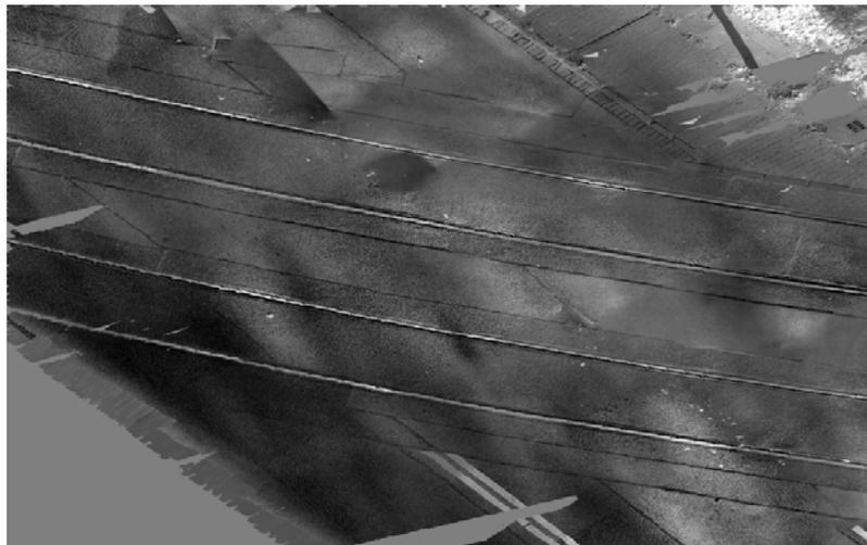
Figure 6.19: Image with a marking, sidewalks, and railways, without cracks (3D-MAPPING 2014).
