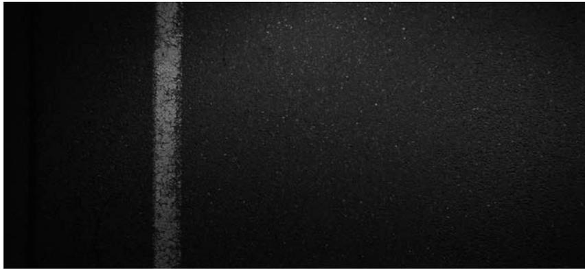
Figure 6.11: Image with moderate pavement texture, and markings with cracks (LEHMANN+PARTNER 2014).
