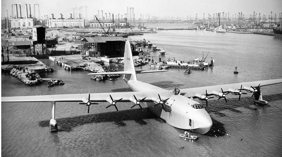
Figure 1.2: Spruce Goose, the largest air plane in history, has a wingspan of 97.5m and is entirely made of wood.
