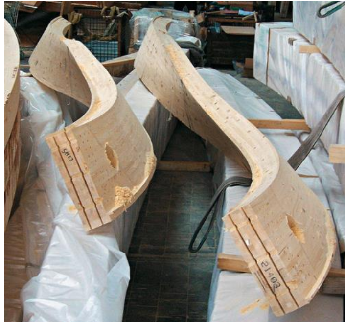
Figure 1.4: Double-curved laminated timbers are produced through steps. First, small linear profiles are laminated together with a nearly correct geometry. Second, the surfaces will be milled out to attain the exact geometry. ( http://resilientwood.tumblr.com/post/129299243257/centre-pompidou-metz )
