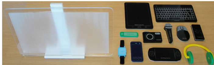
Figure 2.5: Low-fidelity plastic devices created by Chong et al. [CG11] to evaluate how users prefer to spontaneously couple different devices in an ad-hoc manner.
