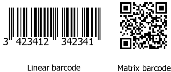
Figure 2.7: This is an example for a linear and matrix barcode.
