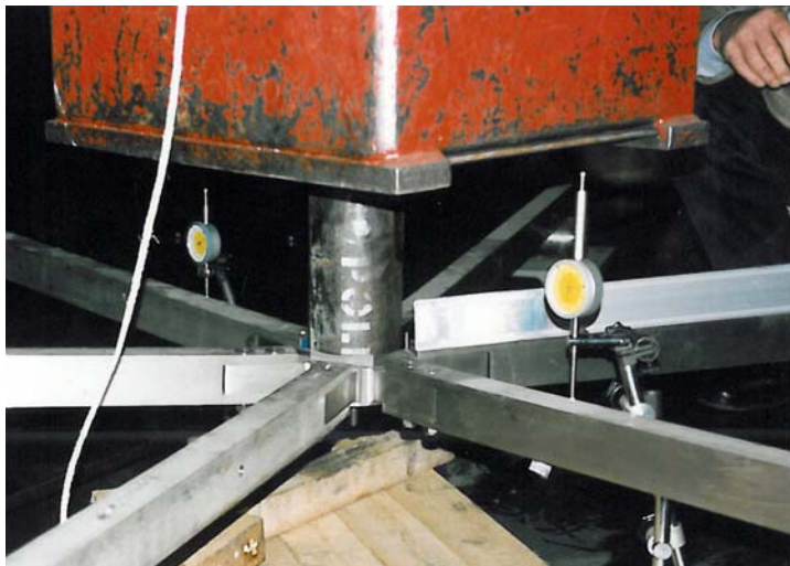
Figure 3.27: View of loading on the center of node and two strain gauges
