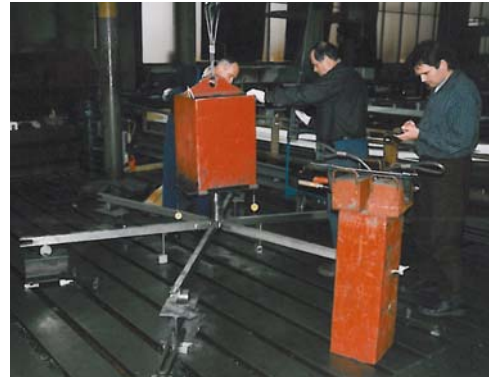
Figure 3.21: Experimental setup of bending test with node connection SBP-3
