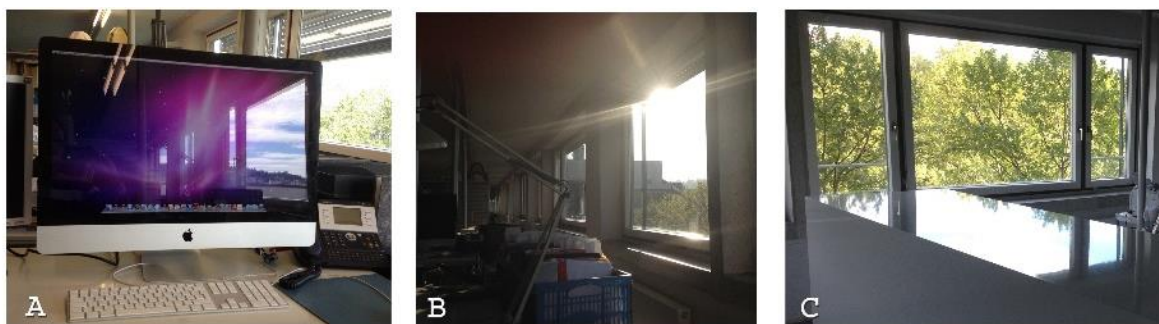
Figure 6 - 11: Direct and indirect glare: (A) Veil reflections on visual display terminal VDT; (B) Direct glare from windows; (C) Indirect glare from glossy surfaces (by researcher)
