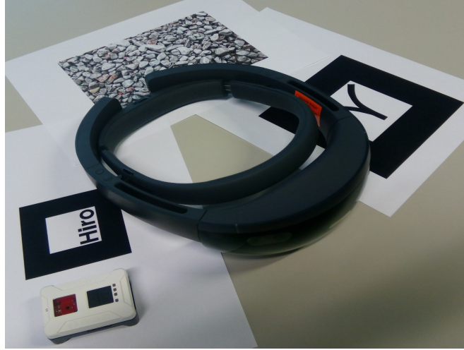
Figure 6.1: Augmented reality glasses, fiducial markers and programmable sensor, used for building the prototype.
