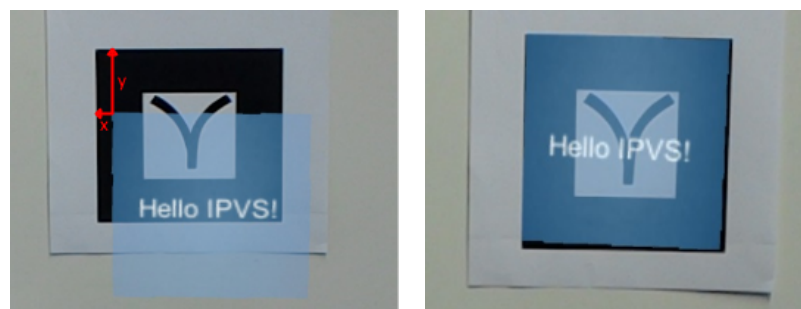
(a) initial pose estimation with offset (b) offset elimination with affine transformation applied
