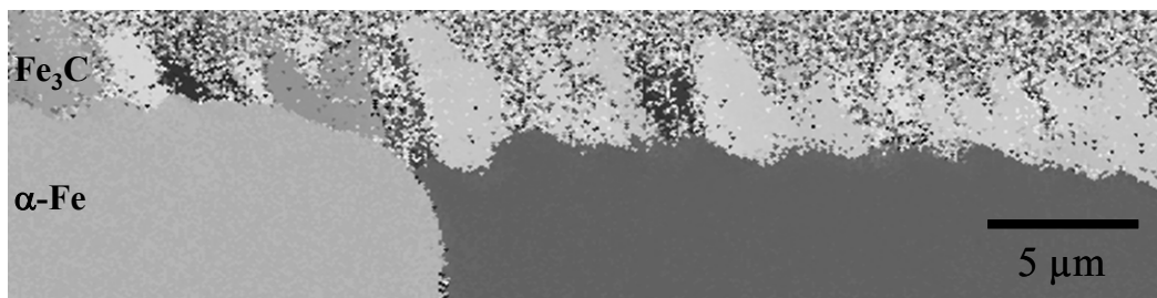
Fig. 4.4: Cross-sectional EBSD image of a ferrite specimen nitrocarburised at 823 K for 48 h using a gas atmosphere containing 13 vol.-% \text{NH}_3 , 58 vol.-% \text{H}_2 , 20 vol.-% \text{CO} and 9 vol.-% \text{N}_2 indicating that on single ferrite-substrate grain several, differently oriented cementite grains grow in a columnar manner (finely dotted areas indicate regions giving rise to insufficiently good Kikuchi patterns from cementite; cf. section 4.2.2).
