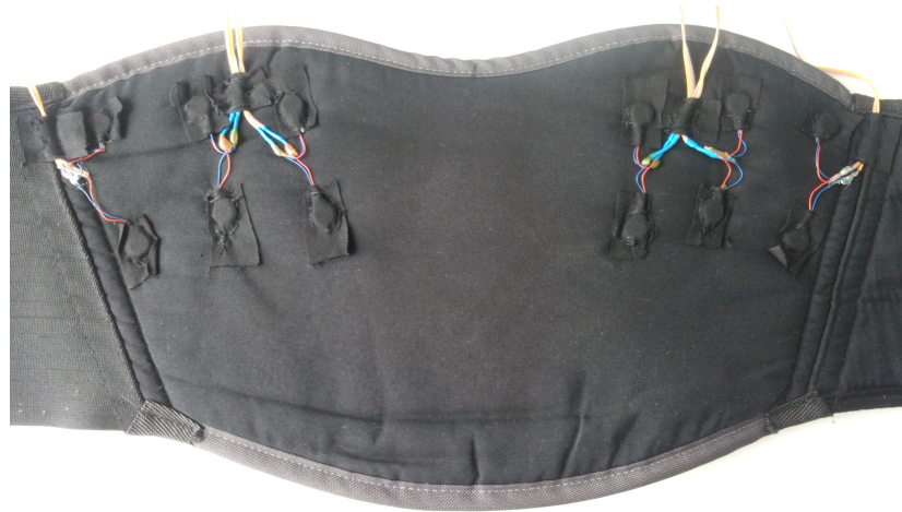
Figure 4.3: Prototype with 3 vibrator pairs on each side.
