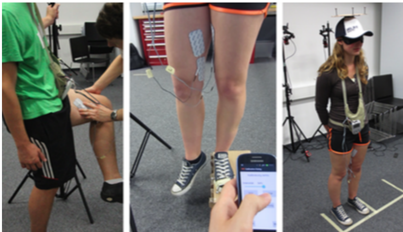
Figure 2.1: The cruise control by Pfeiffer et al. the user is steered in a certain direction by applying a small electrical signal to the inner leg [PDS+15].
