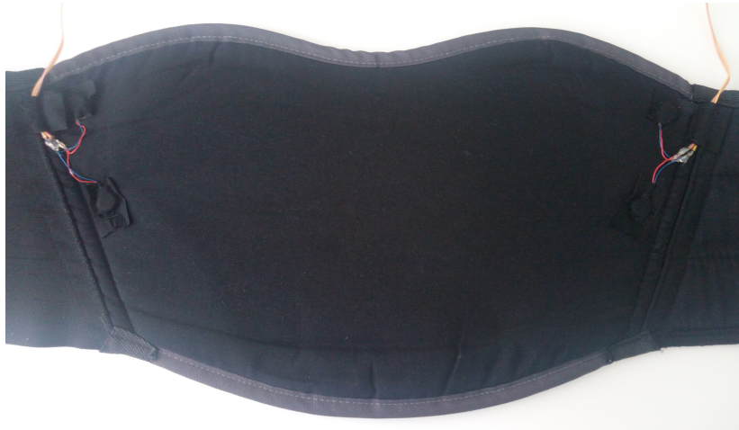
Figure 4.2: Simple vibration pattern prototype featuring four vibration motors
