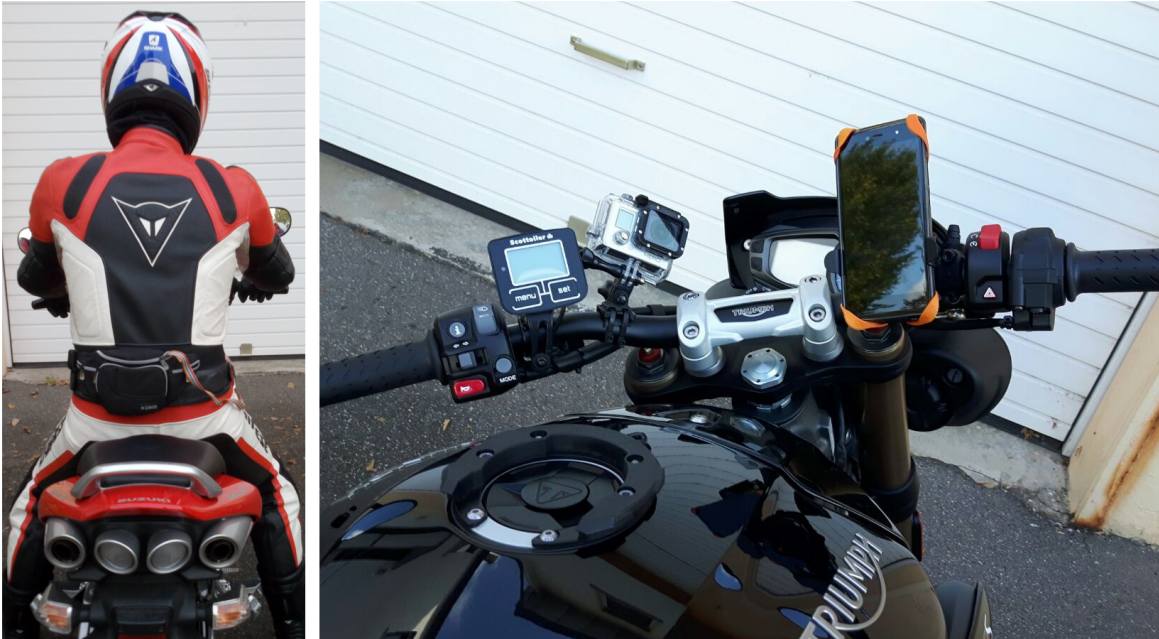
Figure 5.1: The apparatus of the driving study: showing a user wearing the system (left) and the handlebar equipped with a smartphone and a GoPro (right).
