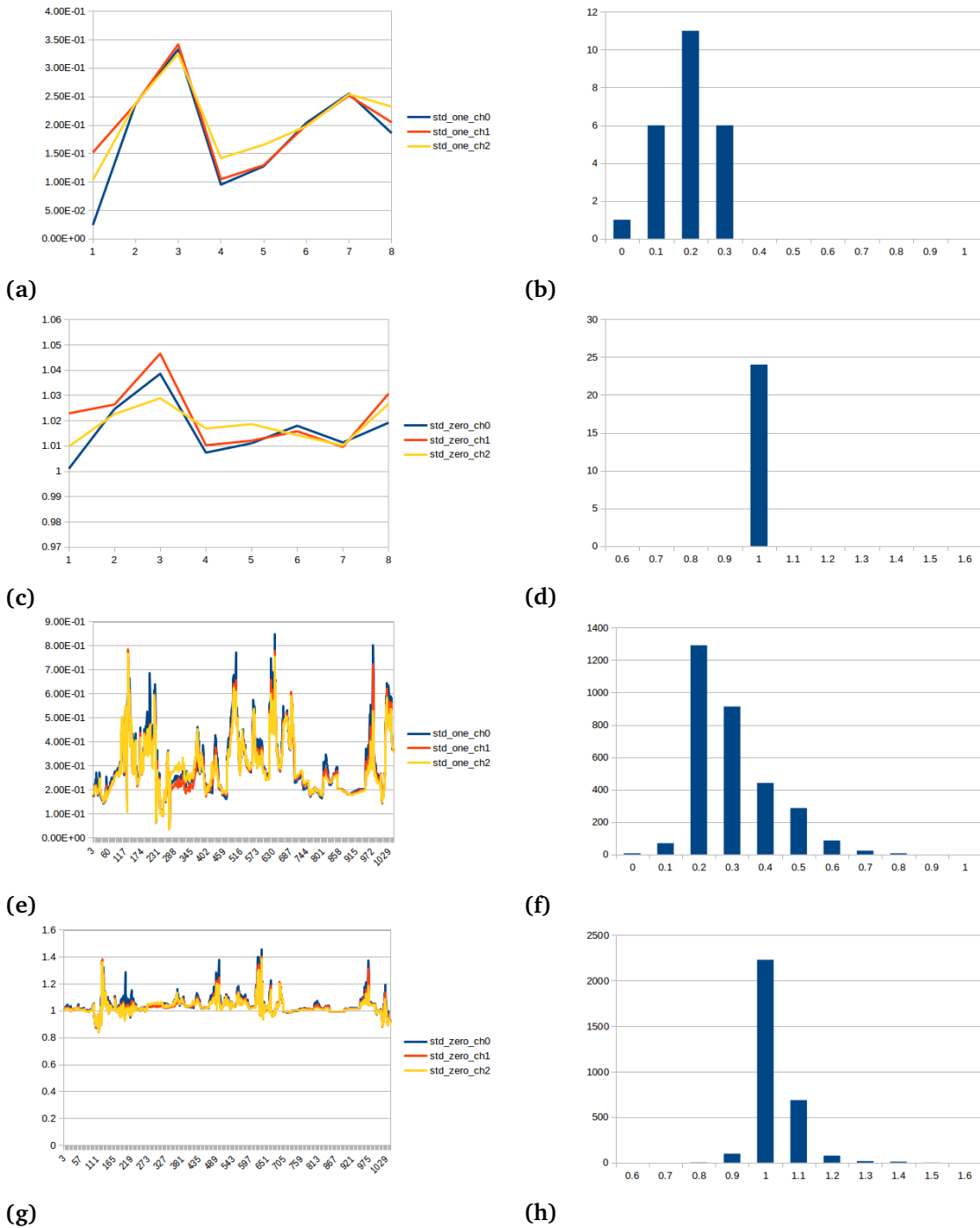
Figure 3.10: STDM and STDA evaluation on the Middlebury and MPI Sintel benchmark (x-axis = frame number) with corresponding histograms in the right column. Middlebury: First row, from left to right: (a) STDM. (b) Histogram of (a). Second row, from left to right: (c) STDA. (d) Histogram of (c). MPI Sintel: Third row, from left to right: (e) STDM. (f) Histogram of (e). Fourth row, from left to right: (g) STDA. (h) Histogram of (g).
