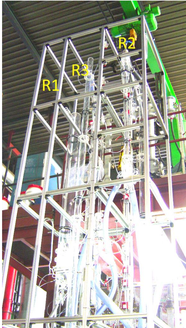
Figure 17 – Cold model set up with the aluminum frame work.
