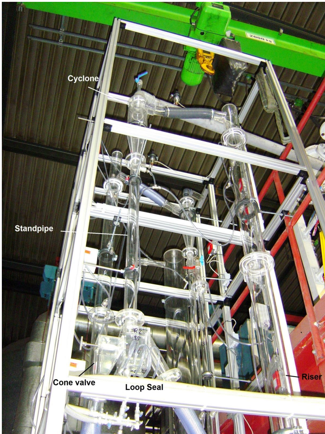
Figure A 3 – Side view of the cold model
