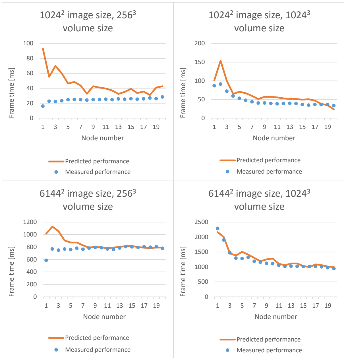
Figure 24: Evaluation of the final model on the validation dataset, which was measured on a different cluster. Best out of three runs, with MSE loss of 5.127 \cdot 10^3 and R^2 score of 0.96.
