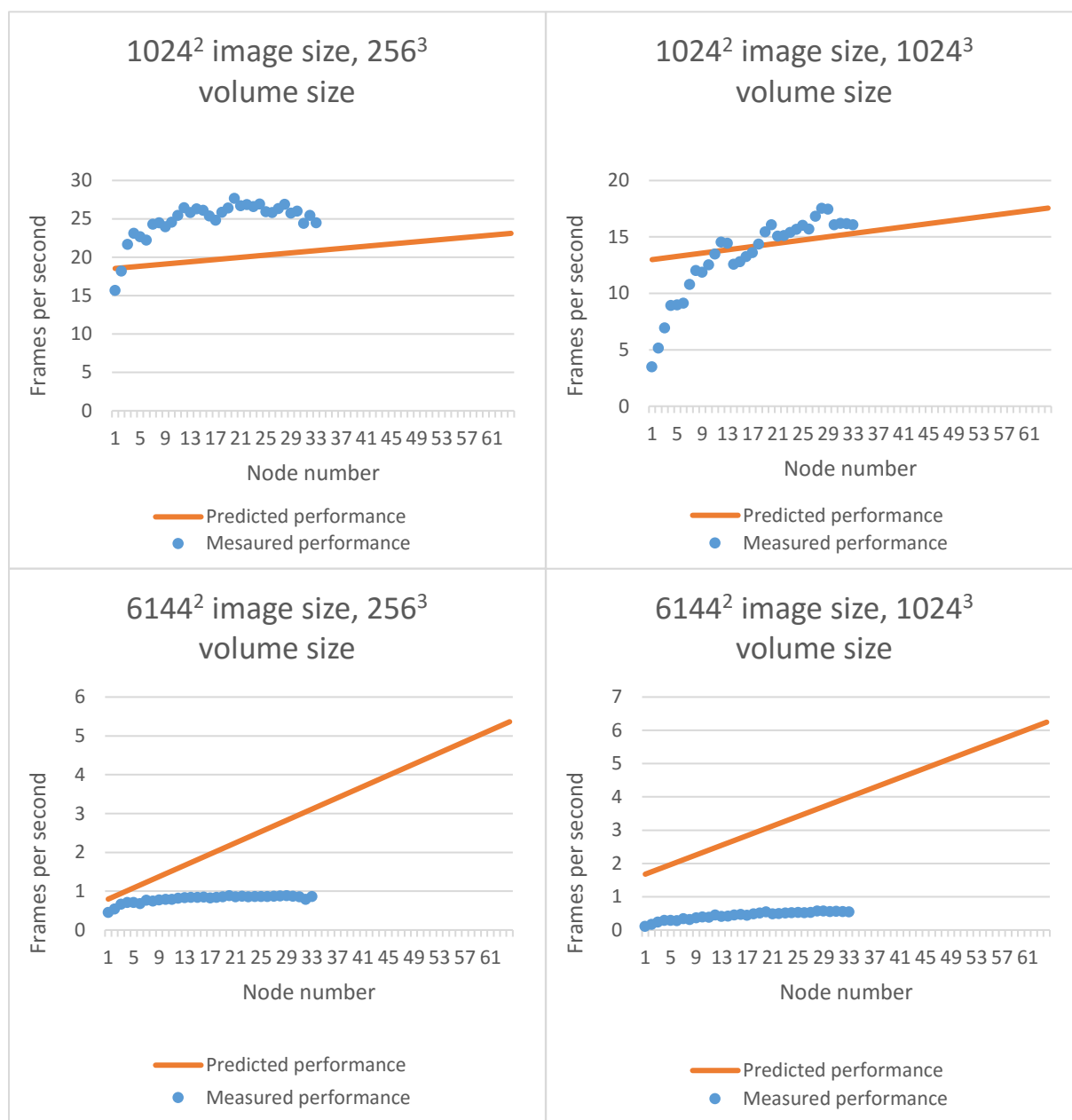
Figure 11: Cluster frames-per-second prediction using linear regression, with additional pixel/voxel number input features.
