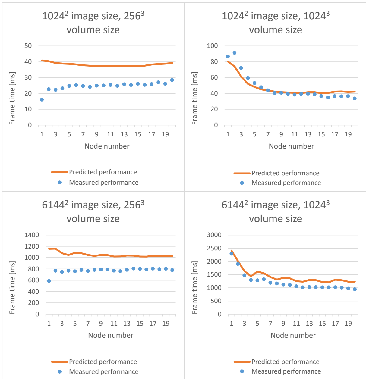
Figure 26: Evaluation of the final model without the 'bin features' of node time histograms, to check if the model utilizes the node time histograms in its prediction. MSE loss of 2.179 \cdot 10^4 and R^2 score of 0.83
