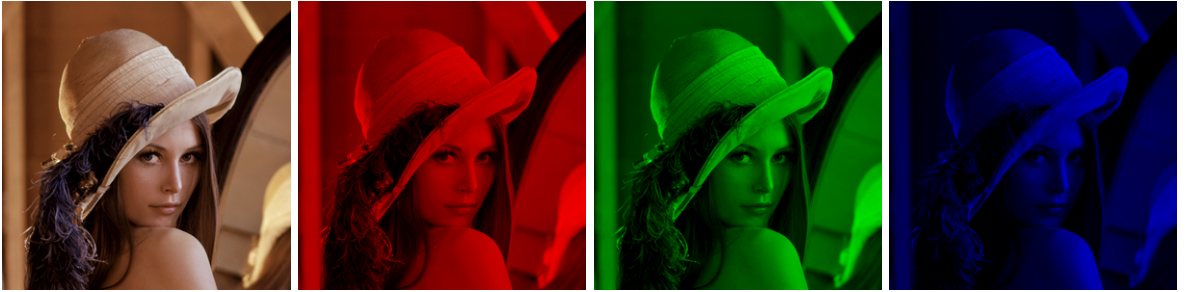
Figure 2.1: RGB image (Lena) and its separate color channels. From Left to Right: Full image, red channel, green channel and blue channel.
