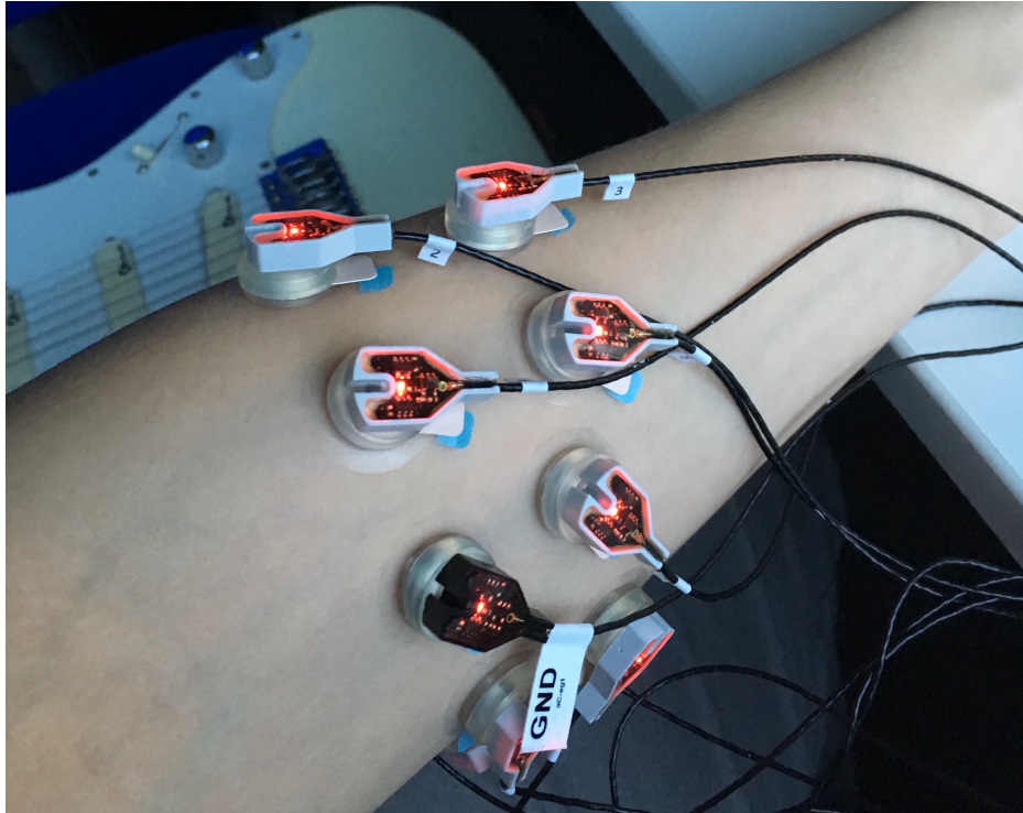
Figure 3.2: Attachment of the electrodes in form of two rings around the upper forearm
