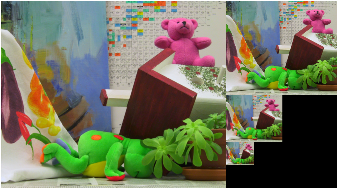
Figure 2.11: A pyramid of 4 levels with \eta = 0.5 constructed using Algorithm 1. Image source: The Teddy sequence from the Middlebury dataset [SS02].
