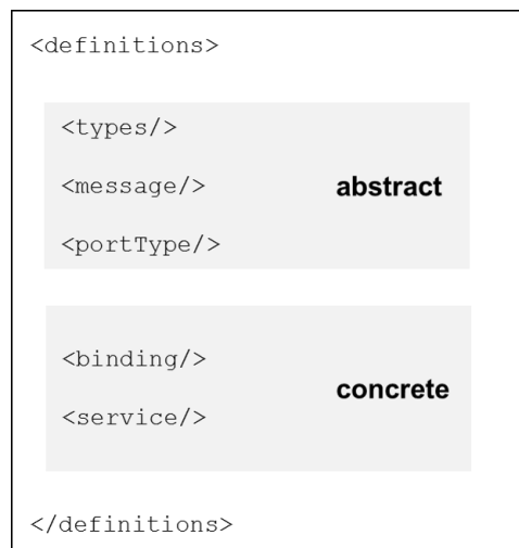
Figure 2.2: The structure of a WSDL (version 1.1) document
