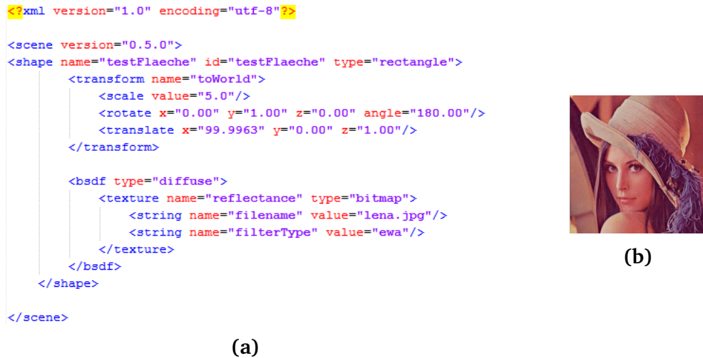
Figure 3.9: An example for a Mitsuba XML scene description file (a) and the corresponding rendering (b). The scene defines a rectangle, its toWorld transformation and its surface properties (A texture from a bitmap file, containing the "lena" picture).
