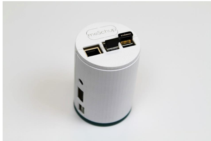
Figure 3.1: A meSchup server in a 3D-printed case.
