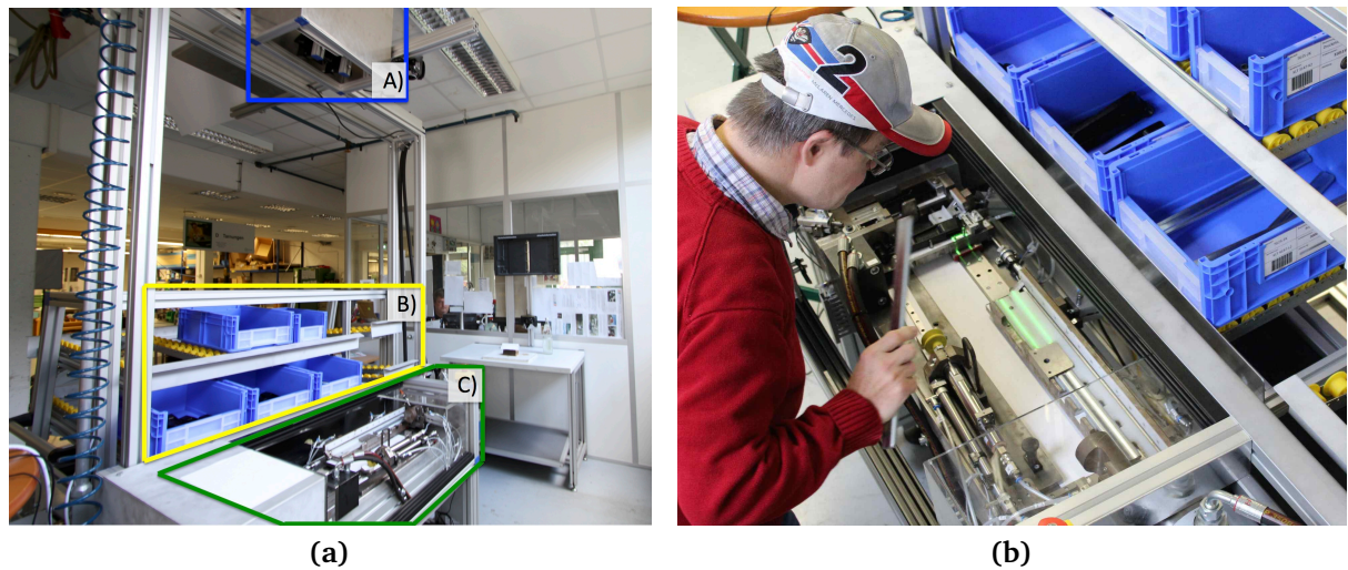
Figure 1.2: (a) Workplace with assistive system (b) providing instructions to the worker with in-situ projection [FBB+15]
