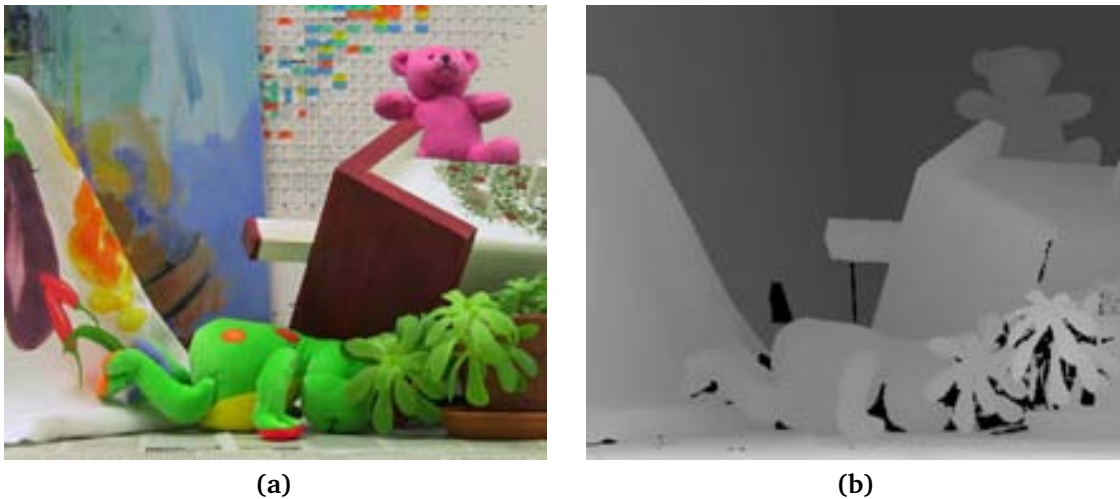
Figure 1.1: (a) Color image of a scene and (b) its corresponding depth image [Sze10]
