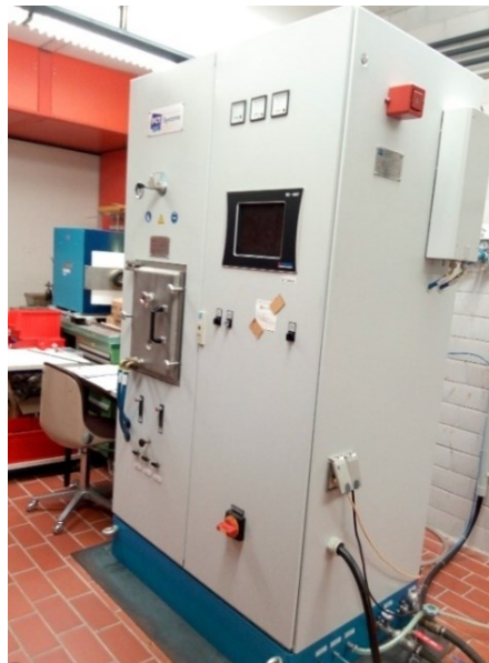
Figure 2-1. Spark plasma sintering (SPS) apparatus used in the experiment in MPI-FKF Stuttgart.
