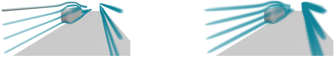
Figure 5.2: Flow over a “blunt body” (front to back). Advection of dye without diffusion model (left, with a streak line for comparison). Active diffusion (right) mimics diffusion of smoke in experimental analysis. Resolution 600 \times 125 \times 121 .
