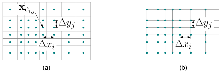
Figure 2.6: Conversion of data representation in rectilinear grids. (a) In a cell-based representation, data values are constant per cell. For conversion to a node-based representation, the data is associated with cell centers c_{i,j} (blue dots). (b) In a node-based representation, data values are stored at grid nodes, and the grid is smaller than the cell-based configuration by half of the cell size on each grid side.
