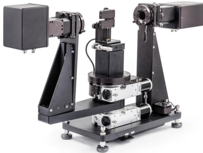
Figure 3. 6: RC2 ellipsometer from J.A. Woollam [64].
