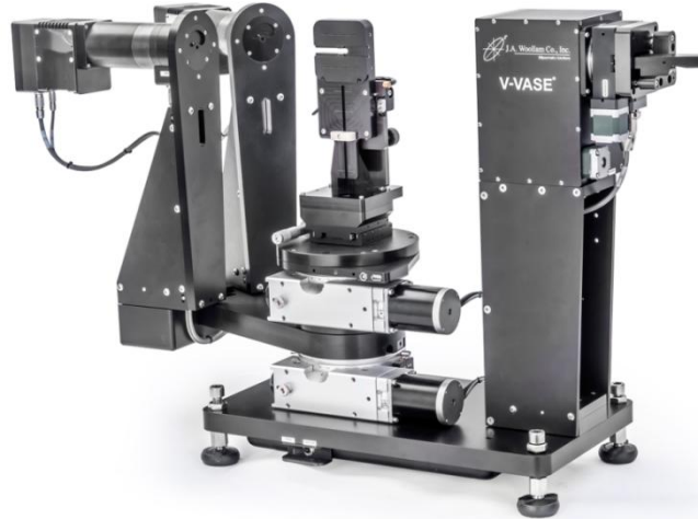
Figure 3. 4: VASE ellipsometer from J.A. Woollam [62].
