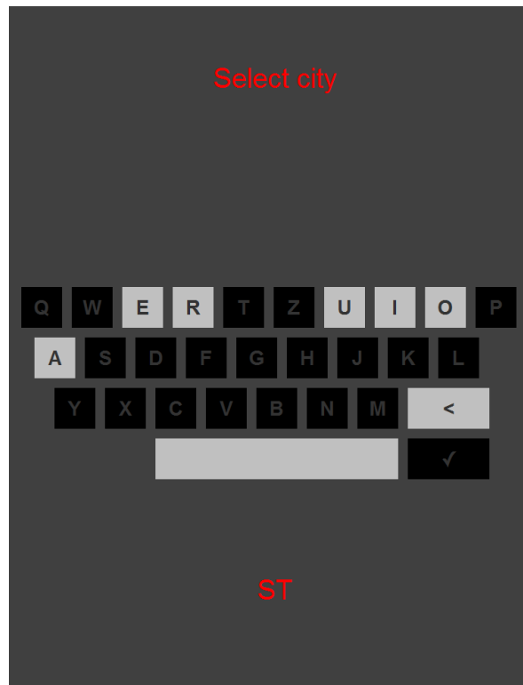
Figure 2.18: The keyboard input method. This method enables the user to search for a location using an onscreen keyboard.
