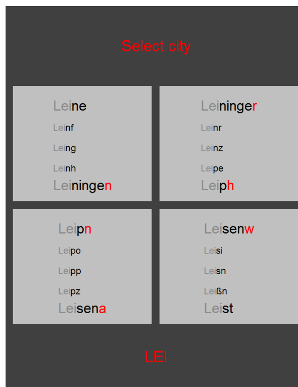
Figure 2.15: The binary input method. The locations are searched for in a quaternary tree.
