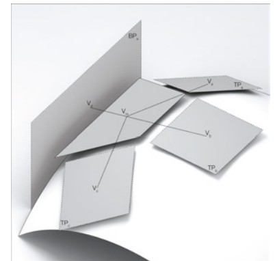
Fig. 4.3.11: The intersection of naked agents with surrounding plate-like agents TP_\alpha , TP_\beta , TP_\gamma and the bounding plane BP_\alpha .
