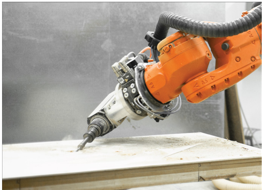
Fig. 4.3.15: The robotic milling process: An interplay between material and fabrication setups; source: Institute for Computational Design and Construction (ICD), University of Stuttgart.
