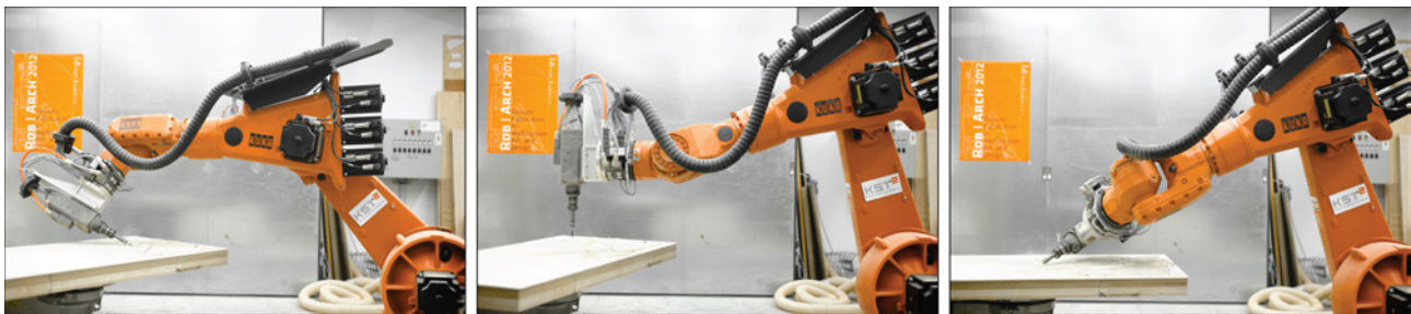
Fig. 4.3.5: The fabrication setup: Milling process of timber plates; source: Institute for Computational Design and Construction (ICD), University of Stuttgart.
