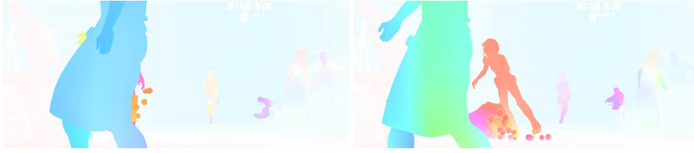
Figure 2.4: Example of constant and affine movement. Left: The person in the foreground has a constant movement to the left since it has nearly everywhere the same colour. Right: The fruits on the ground are rotating which results in an affine movement. [9]
