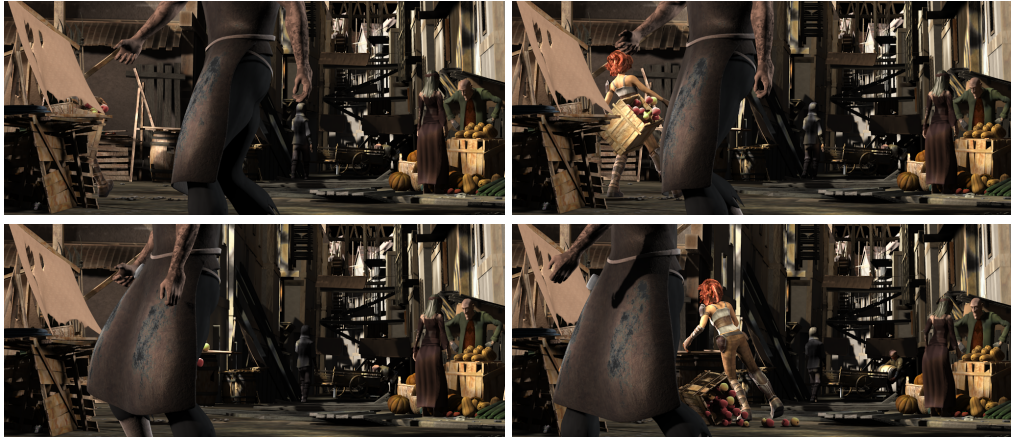
Figure 2.1: Example of occluded pixels. The girl is not yet visible in the first image. She appears in the scenery after some frames where she gets occluded by a person which is passing by. Upper left: Frame 1. Upper right: Frame 5. Lower left: Frame 9. Lower right: Frame 15. [9]
