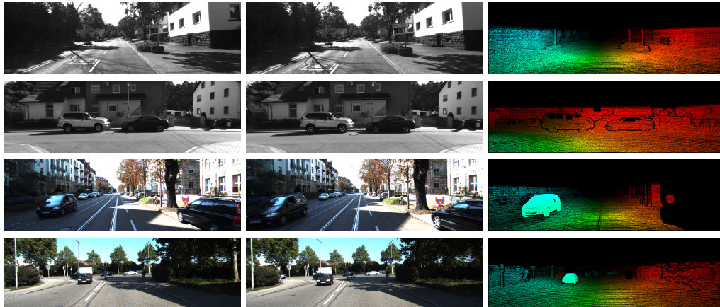
Figure 3.5: Image sequences of the KITTI Vision Benchmark Suite. The two upper rows are from the KITTI 2012 Benchmark while the two bottom rows belong to the KITTI 2015 Benchmark. Left column: First frame. Middle column: Second Frame. Right column: Corresponding ground truth flow. [2], [3]
