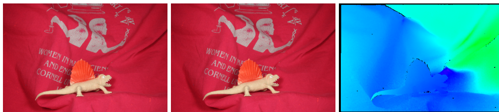
Figure 3.1: An image sequence of the first category of the Middlebury Benchmark where the ground truth flow has been computed via a hidden fluorescent texture. Left: First frame. Middle: Second Frame. Right: Corresponding ground truth flow. [1]
