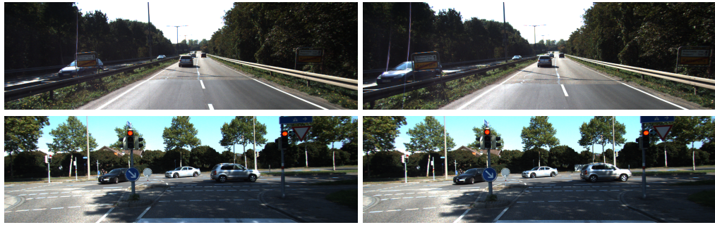
Figure 2.3: Example of occurring illumination effects. Upper row: The car on the left reflects the light such that lens flares appear in the image. Lower row: The white car passing from left to right leaves the shadow in the second frame which results in a brighter appearance. [3]
