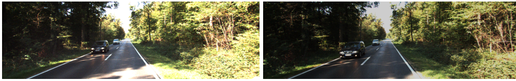
Figure 2.2: Example of illumination change where the second frame is darker than the first one. The second image has been manipulated slightly to demonstrate the effect better. Left: First frame. Right: Second frame. [3]
