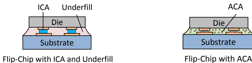
Figure 12 – Flip chip with ECAs
