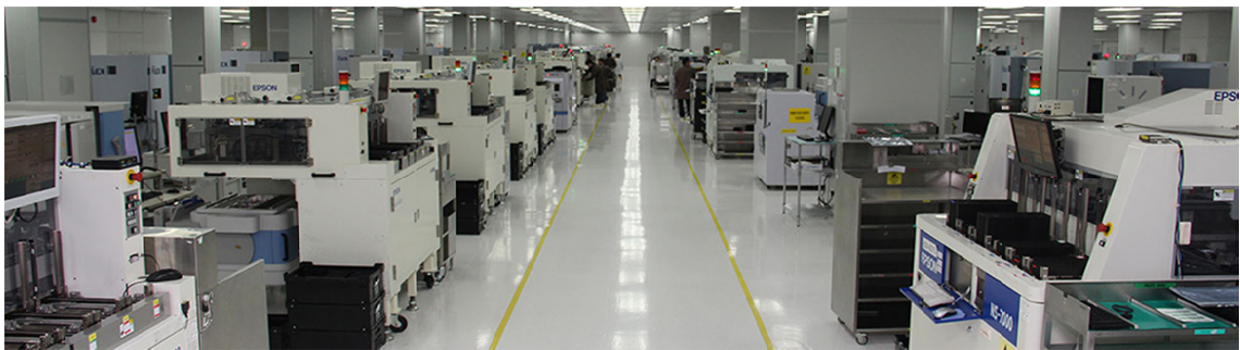
Figure 8 – Sample electronic packaging line (ASE Group 2016)
