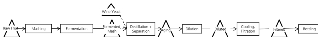
Figure 56: Distillery process chain
