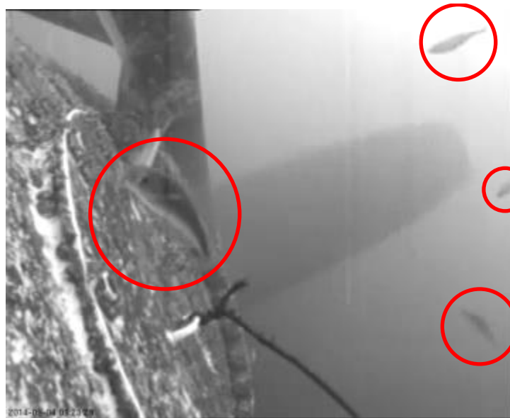
Fig. 2-6: Fish swarm approaching the nacelle of the Voith HyTide ® 1000-13 tidal current turbine at EMEC during operation with n \approx 8.1rpm to feed from the marine growth, [84], Sept. 2014
