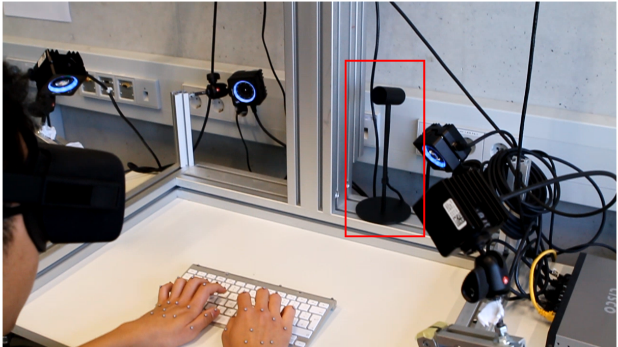
Figure 5.1: A user typing, the Oculus Sensor is highlighted in red
