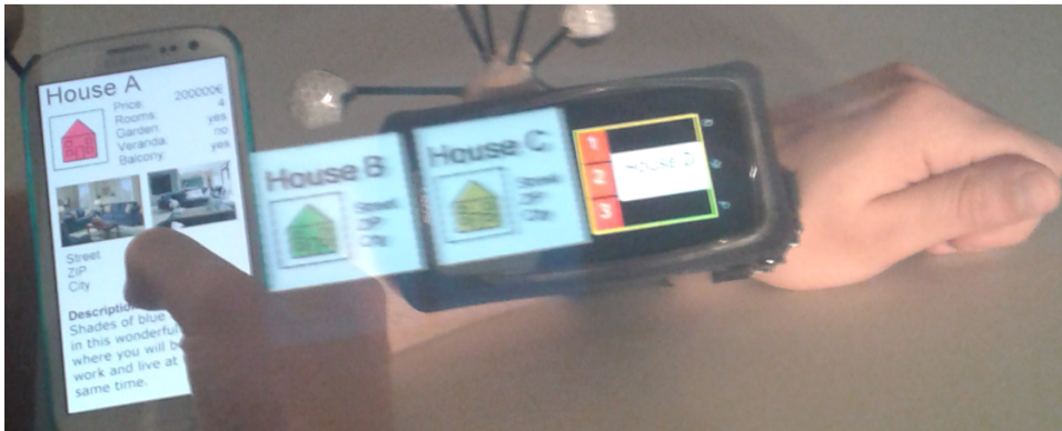
Figure 2.7: MultiFi [GHQS15] combines the strength of using multiple displays by using widgets distributed over multiple devices.
