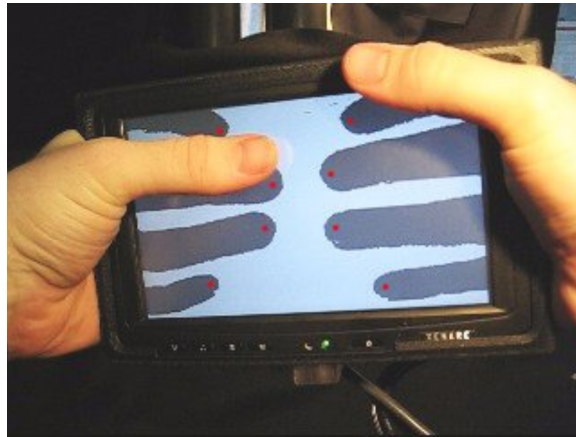
Figure 2.1: LucidTouch [WFB + 07] is a pseudo-transparent device that allows the user to control the device from its backside while still being able to see his hands.
