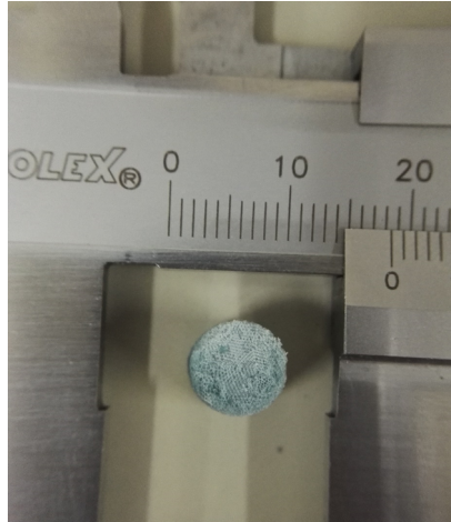
Figure 7.8: Picture of a foam sample used for the determination of the sample's volume with ImageJ.
