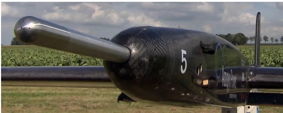
Figure 4.2: Multi-hole probe in an airborne wind energy application [4]
