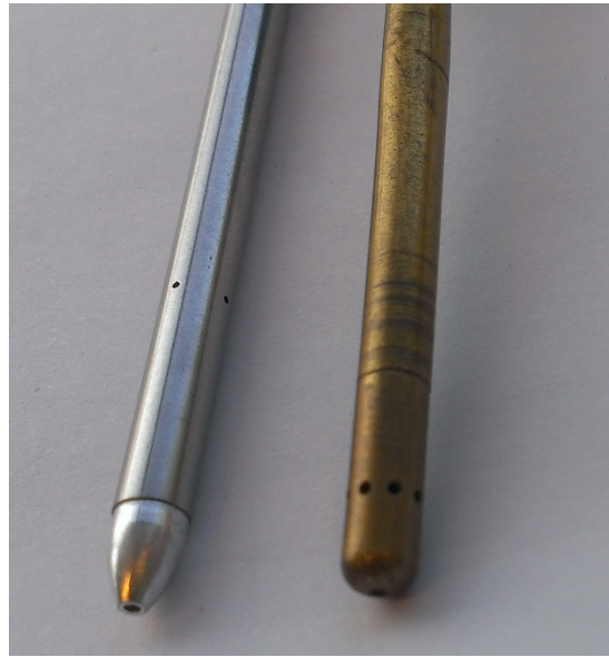
Figure 5.4: New (left) and old (right) Pitot-static tube
