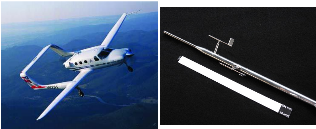
(a) Air data boom on a Adam A500 propeller aircraft (left wingtip) [21] (b) Picture of a miniature air data boom [21]
