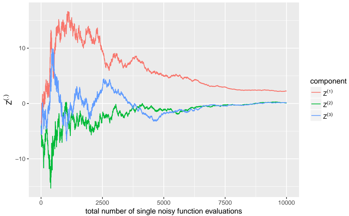
Figure 2.6. The three components of a simulated path of a one-measurement procedure with dependent perturbation and a_n = 2/(200 + n)
