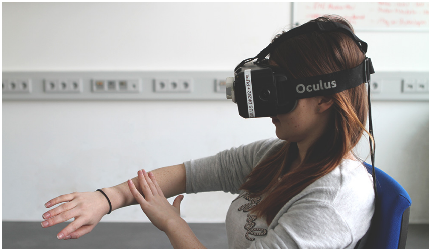
Figure 6.2: User in our VR apparatus: A leap motion sensor for hand tracking and an Oculus Rift DK2 HMD as virtual reality display.
