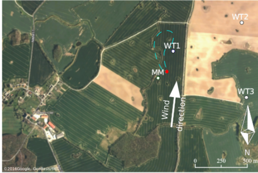
Figure 2: Overview of the test site during this experiment with the three wind turbines (WT1-3) and the met mast (MM), the flight path (dashed cyan line), the measuring location (red dot) and the main wind direction (white arrow).
