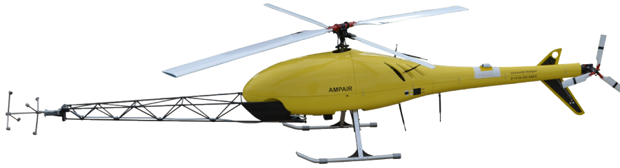
Figure 1: Flightsystem AMPAIR with installed boom and ultrasonic anemometer at the nose.
