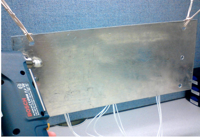
Figure 4.9: Harmonic excitation of the aluminium plate with an electric screwdriver. Sensors are on the back side for this experiment.
