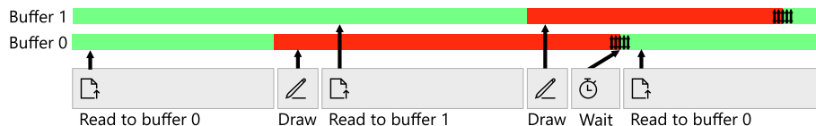
Fig. 1 Simplified illustration of streaming particle data to a persistently mapped buffer, in this case, for two segments. A buffer is marked red while the GPU is rendering on it and green while it is ready to accept new data from the CPU. After the draw call, a fence is injected into the command stream of the GPU, which the GPU will signal once it is done rendering the segment. When the CPU submits the second segment, the GPU uses both buffers simultaneously. Therefore, the next segment cannot be uploaded, and the CPU needs to wait for the GPU to finish work. This can be achieved by waiting for the fence to be signalled. In the actual implementation, the CPU does not wait for a specific buffer to become ready but for any of them
