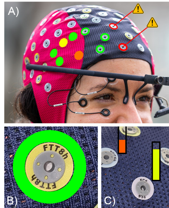
Fig. 26: Examples of possible visualizations. A) several types including the notification pin. B) the current version, which consists of a ring around the electrode that changes color depending on the impedance value. C) a bar that fills up and changes color depending on the impedance value.
