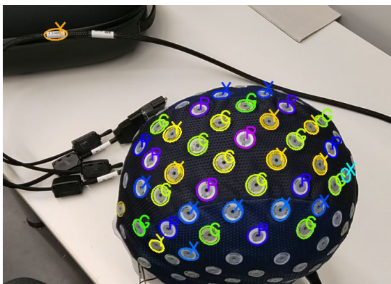
Fig. 11: Detection of electrodes with contour detection and fitEllipse(...) method of OpenCV. Detected electrodes are marked with their detected color. Letters near each electrode indicate classified color.
