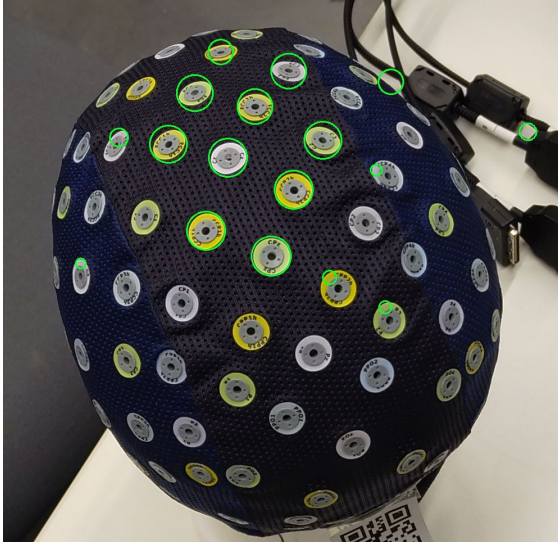
Fig. 7: Detection of electrodes by using contour detection and minimum enclosing circles around contours to detect circles in the preprocessed image. Detected circles are marked green.
