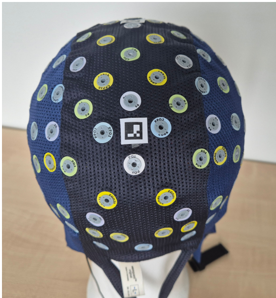
Fig. 24: Image of an ArUco marker placed at the predefined position between electrodes on the EEG cap.
